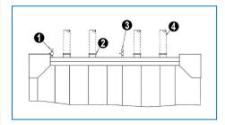
End elevation - Air vents on TSU-237M and TSU-L184M
