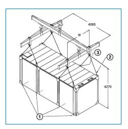
Recommended rigging method for 6 m long units
