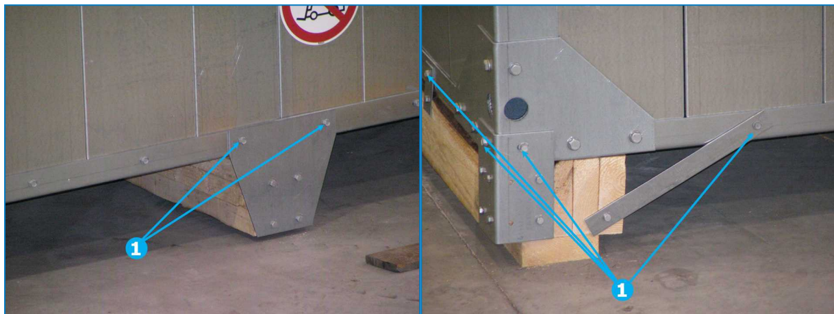
Removal of shipping skids – Side view & End view
