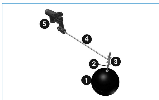
Water make-up valve assembly
