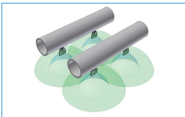
Nozzle spray distribution type for condenser
