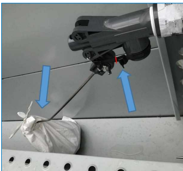
Fixation and wrapping of float ball
