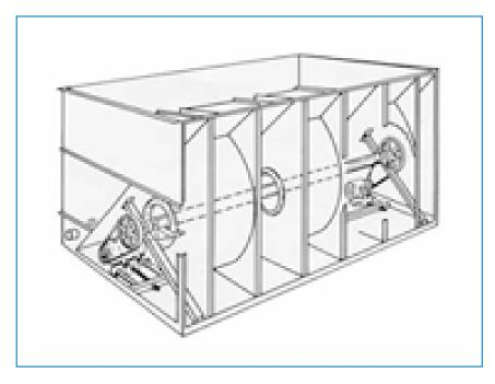
The installation of a Baltiguard<sup>®</sup> Drive System
