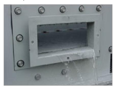
A factory-installed clean out port
