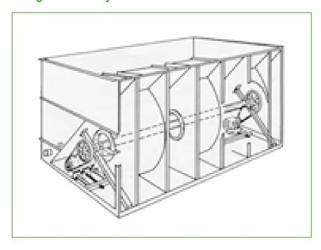
The installation of a Baltiguard  $^{\! ^{^{\rm \tiny B}}}\!\!$  drive system
