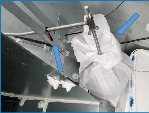
Fixation and wrapping of Float ball
