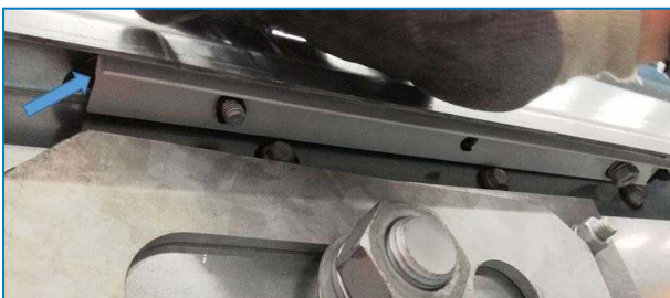
Installed sealing profile
