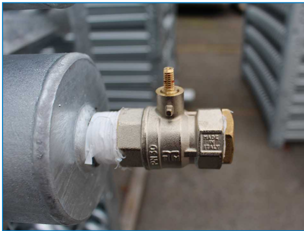
Upper coil connection with pressure release valve on closed circuit cooling towers with connections bigger than ND100.
