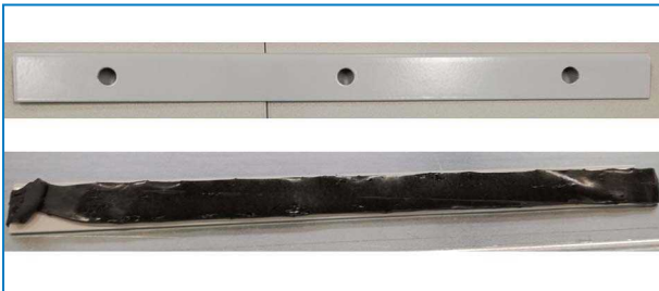
Sealing profile with butyl sealer
