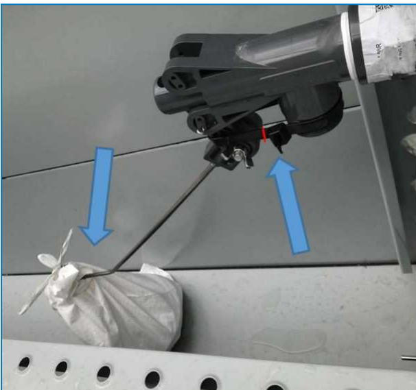
Fixation and wrapping of float ball
