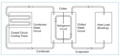
Figure 2 : Chiller Loop with Closed Circuit Tower
