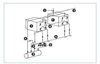
Figure 10: Parallel Evaporative Condensers with Common Liquid Header Above Receiver Level: Alternate 1 1. Condenser; 2. Receiver; 3. Discharge Line from Compressor; 4. Equalizing line; 5. Common Liquid Header; 6. Liquid Line to Evaporator; 7. Alternate Purge Valve when Unit Shut Down (See Purging); 8. Purge Valves (See Purging); 9. Relief Valve; 10. Pump Out Valve; 11. Charging Valve
