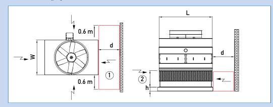
Figure 6: Unit with Four Air Inlets adjacent to a Wall 1. Envelope Area; 2. Air Intake Height
