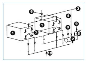
Figures 10 and 11(Parallel Evaporative Condensers with Common Liquid Header above Receiver Level: Alternate 1 and Alternate 2) show two recommended piping methods for multiple condensers with top inlet receivers. These two methods are equally acceptable and will give the same results.
