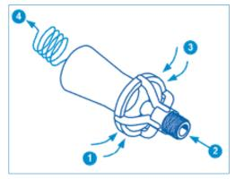
Figure 5: Eductor 1. Sweeping: Circulate four Litres of Sump Water; 2. One Litre of Filtered Water from Pressure Line; 3. Eductor; 4. Five Litres Circulated
