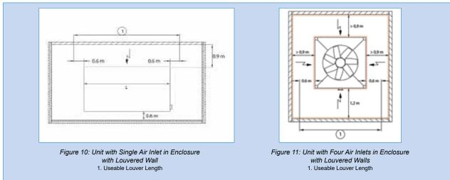
Therefore, louver sizing is sufficient because 2,6 m/s < 3 m/s maximum allowable. The same procedure as described above, can be followed in order to determine whether the layout meets the requirements for a louvered well installation.
