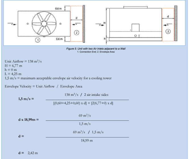
This is rounded up to the next 0,1 m increment. Therefore, the air intake should be located no less than 2,5 meter from the solid wall.
