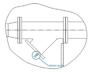
Example of a connection at right angle of the tube end. The length of the main piping should be as short as possible after the connection to avoid a dead end pipe.
