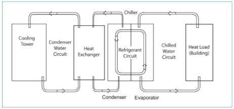
Figure 3 : Chiller Loop with Open Tower/Heat Exchanger Combination
