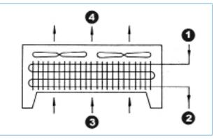
Figure 5: Air-Cooled Condenser 1. Refrigerant Vapor In; 2. Refrigerant Liquid Out 45°C; 3. D.B. Inlet Air 35°C (130 l/s : 1kW); 4. Air Discharge
