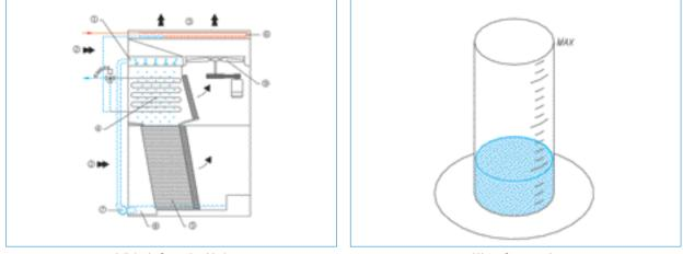
Adiabatic Operation Mode 1. Water Distribution System; 2. Air In; 3. Air Out; 4. Prime Surface Coil; 5. Wet Deck Surface; 6. Finned Coil; 7. Spray Pump; 8. Sump; 9. Axial Fan.
