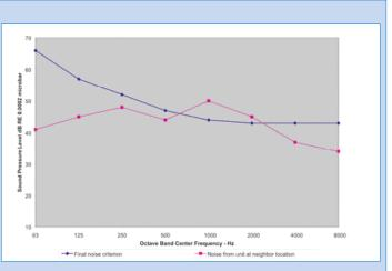
Figure 5: Comparison of Final Noise Criterion and Equipment Sound Levels
