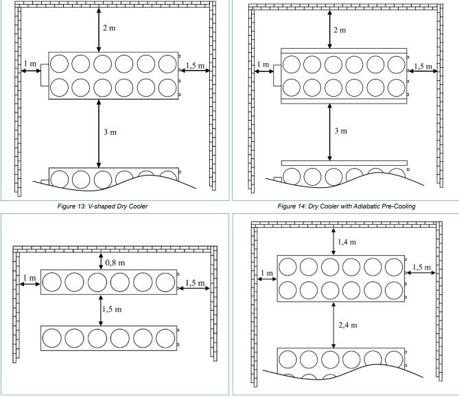
Figure 15: Horizontal Dry Cooler - single row fans
