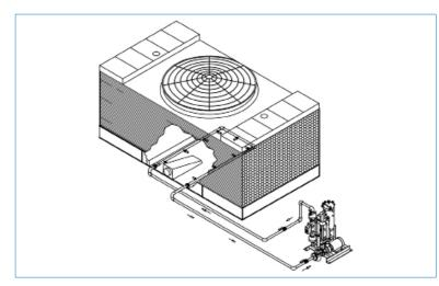
Figure 6: Filtration System with Sump Sweeper Piping
