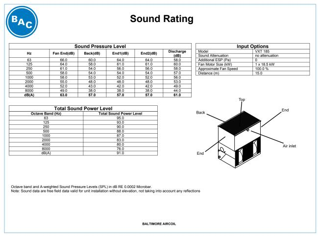
In addition to the five sets of sound pressure levels at each of the two distances, the data sheets contain the calculated sound power level values for the reference power level 10<sup>-12</sup> watt. Current sound data for all BAC equipment is available from BAC Balticare Representative.
