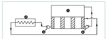
Figure 15: Auxiliary Cooling using Condenser Pan Water 1. Evaporative Condenser; 2. Cooling Load; 3. Auxiliary Pump; 4. Standard Condenser Pump
