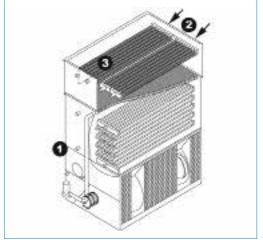
Figure 13: Evaporative Condenser with Desuperheater Coil 1. Liquid Outlet; 2. Hot Gas from Compressor; 3. Desuperheater Coil
