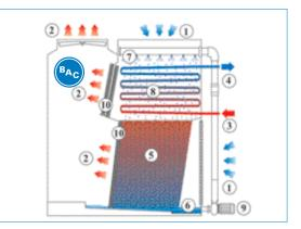
Closed Circuit Cooling Tower 1.Air in; 2. Air out; 3. Fluid in; 4. Fluid out; 5. Wet Deck Surface; 6. Cold Water Basin; 7. Water Distribution System; 8. Coil; 9. Spray Water Pump; 10. Eliminators.
