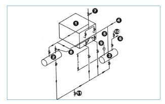
Figure 12: Paralleling an Evaporative Condenser and a Shell & Tube Condenser
