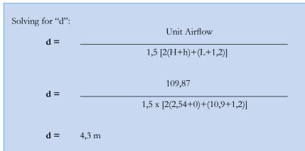
Therefore, the air intake should be no less than 4,3 meter from the wall.
