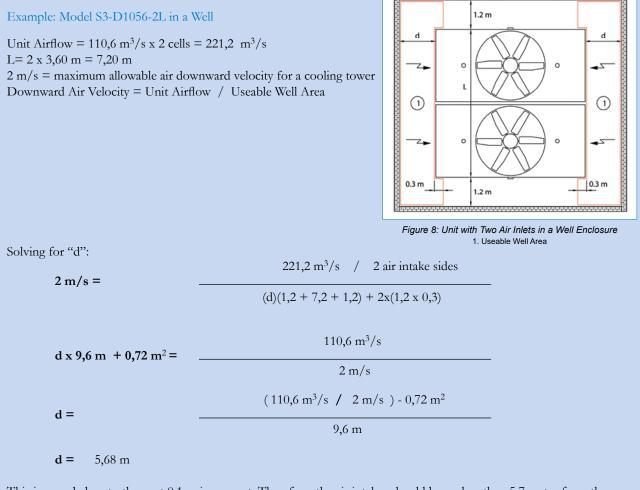
This is rounded up to the next 0,1 m increment. Therefore, the air intakes should be no less than 5,7 meter from the enclosure walls.
