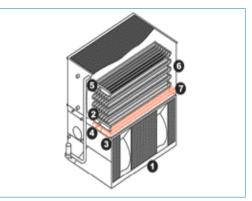
Figure 14: Evaporative Condenser with Liquid Subcooling Coil 1. Evaporative Condenser; 2. Refrigerant Liquid Outlet to Receiver; 3. Inlet Subcooling Coil coming from Receiver; 4. Subcooled Liquid from Subcooling Coil to Expansion Valve; 5. Compressor Discharge; 6. Condensing Coil; 7. Subcooling Coil.
