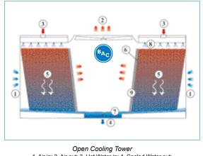
1. Air in: 2. Air out: 3. Hot Water in: 4. Cooled Water out: 5. Water; 6. Wet Deck Surface; 7. Cold Water Basin; 8. Water Distribution system; 9. Eliminators
