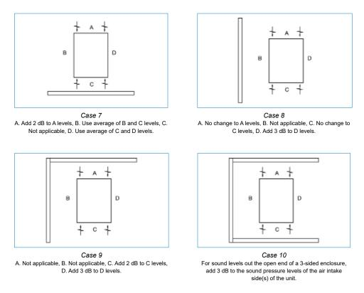
These figures and their associated adjustment values are to be used to correct base 15 m sound pressure level ratings in the neighbour direction of the effect of the reflecting surface conditions shown.
