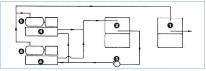
Figure 16: Evaporative Condenser with Closed Circuit Evaporative Cooler for Fluid Cooling: Cooling Oil for Refrigeration Screw Compressors 1. Evaporative Condenser; 2. Closed Circuit Evaporative Cooler; 3. Pump; 4. Oil Cooler; 5. Screw Compressor
