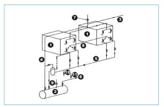
Figure 11: Parallel Evaporative Condensers with Common Liquid Header Above Receiver Level: Alternate 2 1. Condenser; 2. Receiver; 3. Discharge Line from Compressor; 4. Equalizing line; 5. Common Liquid Header; 6. Liquid Line to Evaporator; 7. Alternate Purge Valve when Unit Shut Down (See Purging); 8. Purge Valves (See Purging); 9. Relief Valve; 10. Pump Out Valve; 11. Charging Valve
