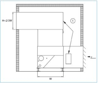
Figure 12: Ducted Unit Enclosure 1. Access Doors
