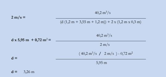
This is rounded up to the next 0,1 m increment. Therefore the air intake should be no less than 3,3 meter from the enclosure walls.
