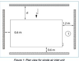
gure 1: Plan view for single air inlet unit 1. Connection end
