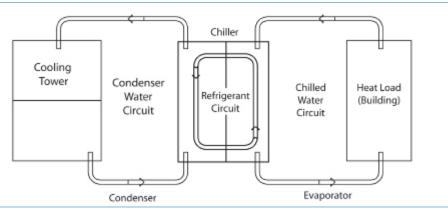
Figure 1 : Chiller Loop with Open Tower
