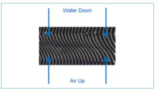
Crossflow Configuration (open cooling towers only)
