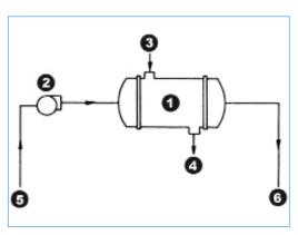
Figure 3: "Once-Through" Condensing Systems
