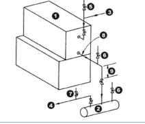
Figure 7: Single Evaporative Condenser with Top Inlet Receiver 1. Evaporative Condenser; 2. Receiver; 3. Compressor Discharge Line; 4. Liquid Line to Evaporator; 5. Alternate Purge Valve when Unit Shut Down; 6. Purge Valve; 7. Charging Valve; 8. Slope 22 mm/m toward Receiver; 9. 300 mm minimum.
