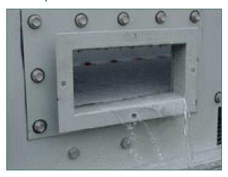
A factory-installed clean out port
