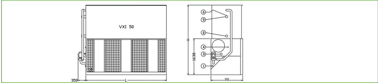
1. Drain ND50; Outlet connection ND100; 3. Overflow ND80; 4. Make up ND25; 5. Inlet connection ND100; 6. Vent ND15; 7. Access door.
