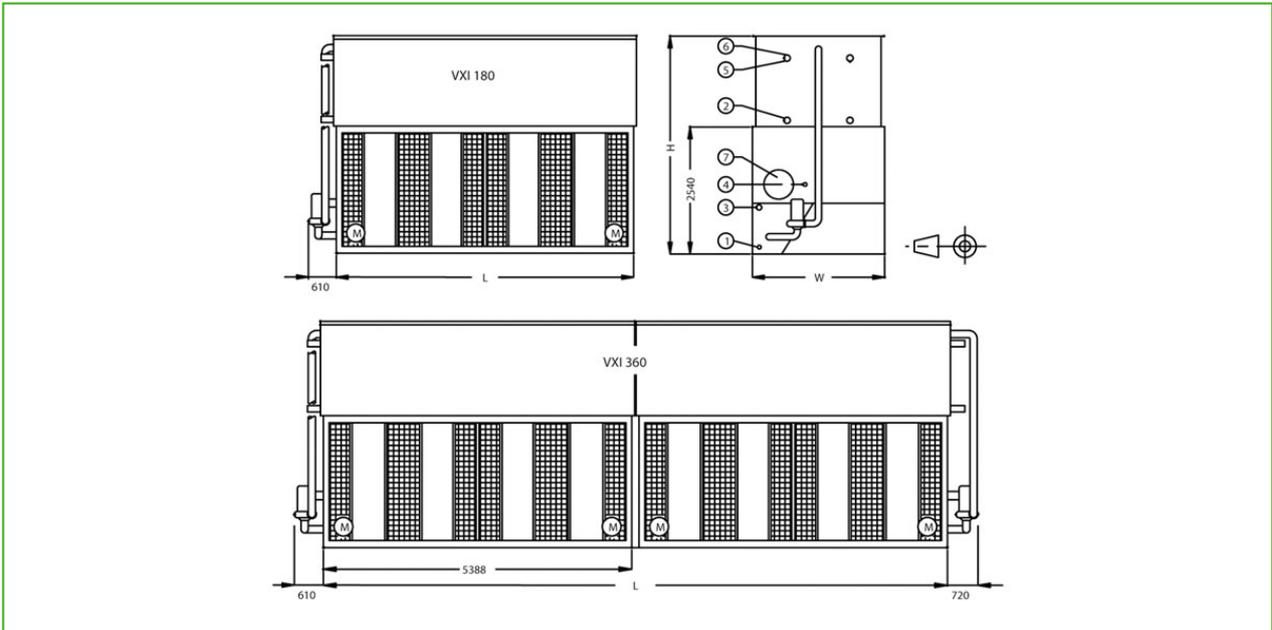
1. Drain ND50; 2. Outlet connection ND100; Overflow ND80; Make up ND50 for VXI 180-X and ND80 for VXI 360-X; 5. Inlet connection ND100; 6. Vent ND15; 7. Access door.
