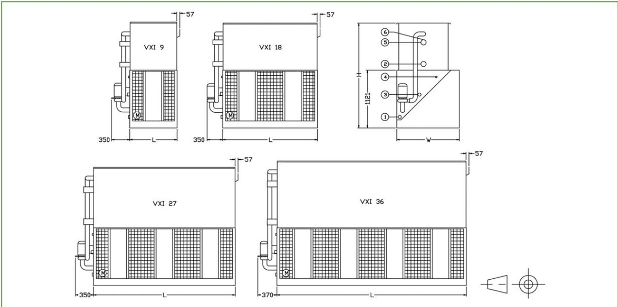
1. Drain ND50; 2. Outlet connection ND80 for VXI 9-X and ND100 for VXI 18-X, 27-X and 36-X; 3. Overflow ND50; 4. Make up ND25; 5. Inlet connection ND80 for VXI 9-X and ND100 for VXI 18-X, 27-X and 36-X; 6. Vent ND15; 7. Access door (not shown).
